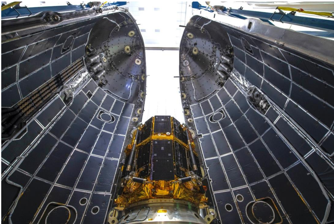
ispace's M1 lunar lander integrated into the SpaceX Falcon 9 fairing.
