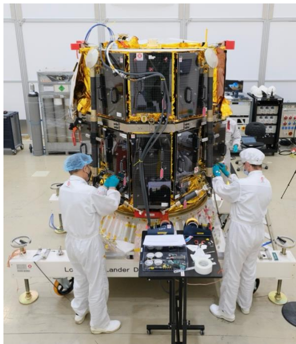
ispace engineers assembling the M1 flight model at the IABG GmbH Space Centre in Germany.
