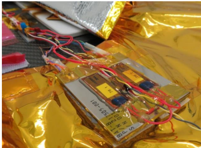
(Above: NGK Spark Plug's solid-state battery test module integrated into ispace's lander.)
