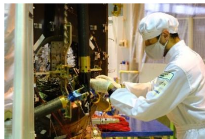
Above: ispace engineers conduct testing on the structure thermal model of the HAKUTO-R lunar lander.
