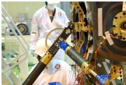
Above: ispace engineers conduct testing on the structure thermal model of the HAKUTO-R lunar lander.
